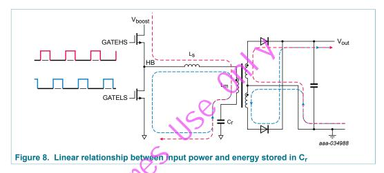
When the high-side switch is on, a primary current is flowing through the transformer and resonant capacitor  $C_r$  as indicated by the red line. Half the energy the input delivers is transferred to the output. The other half charges resonant capacitor  $C_r$ . The voltage across the resonant capacitor increases.
